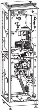
Connect the exhaust air hose and suction hose to the floor connection.
