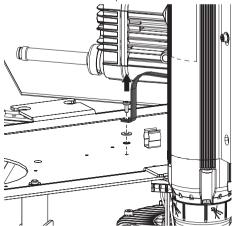
> Remove the clip for L bracket.
