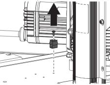
> Mount the valve block with earth strap.
