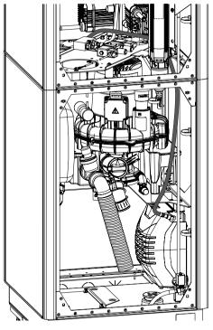
Lay the valve cable from the valve block to the PCB.
