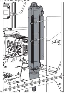
Insert nozzle, see installation instructions 9000-610-49/01. Insert the filter and close the drying unit with the cover.
