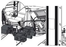
Establish the compressed air connection between the compressor unit and valve block.
